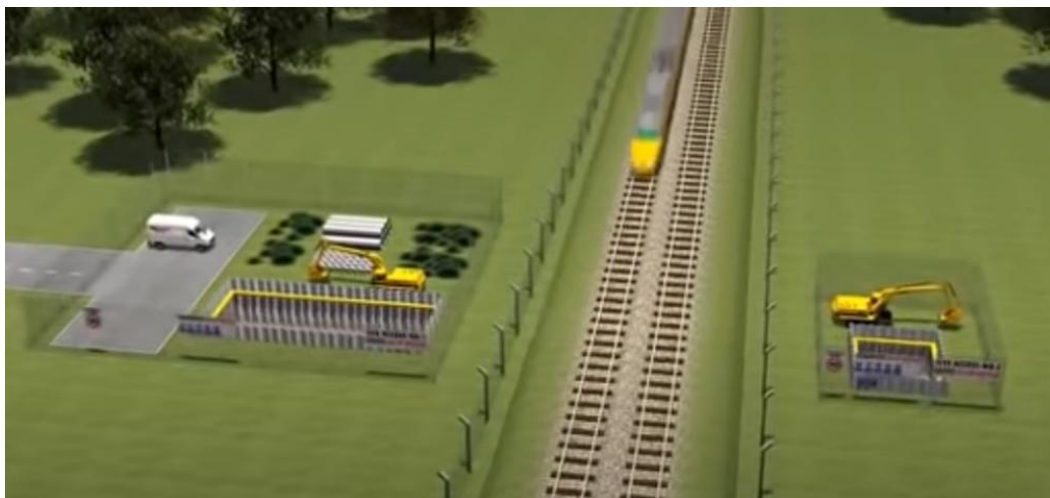
Figure 38 - Typical Auger-boring Set Up for Deep Crossing
