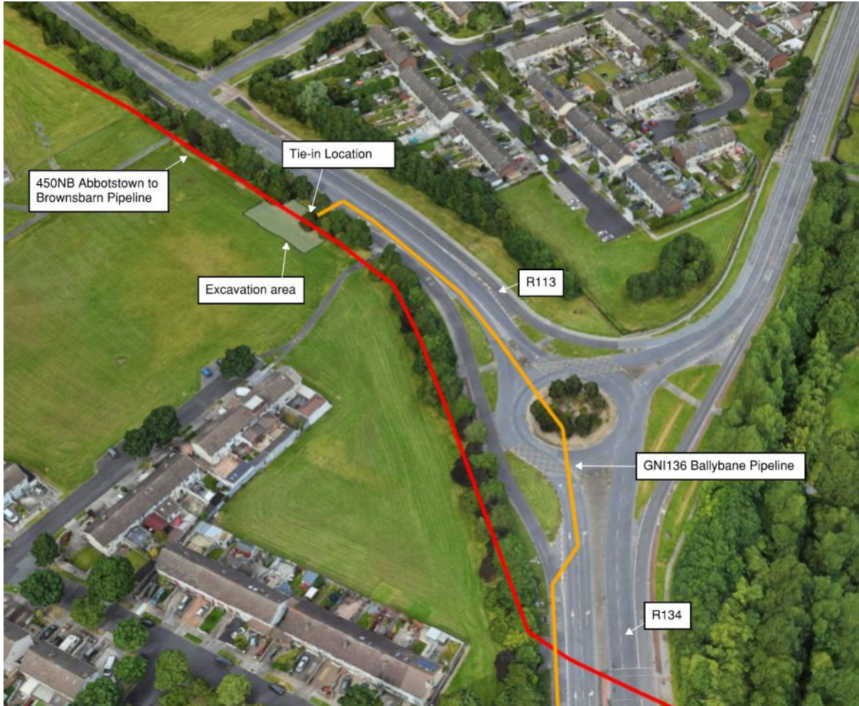
Figure 23 - Tie-in location 3D view
