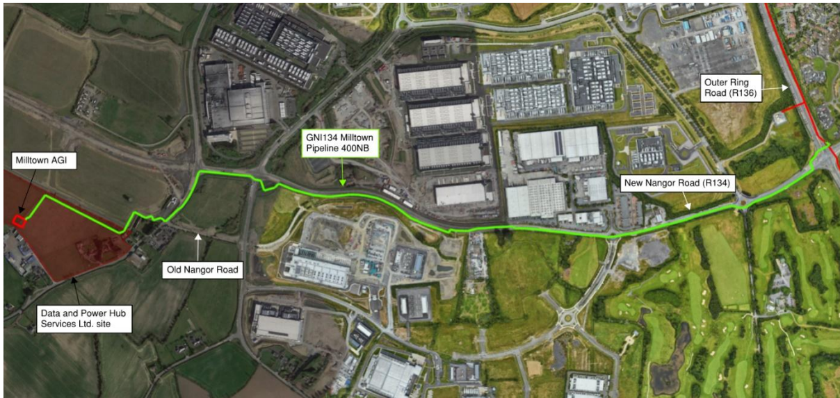
Figure 2 - Overview of Data & Power Hub Services Site, GNI134 Pipeline Route, AGI Location, and Location of Nearby Transmission Network
