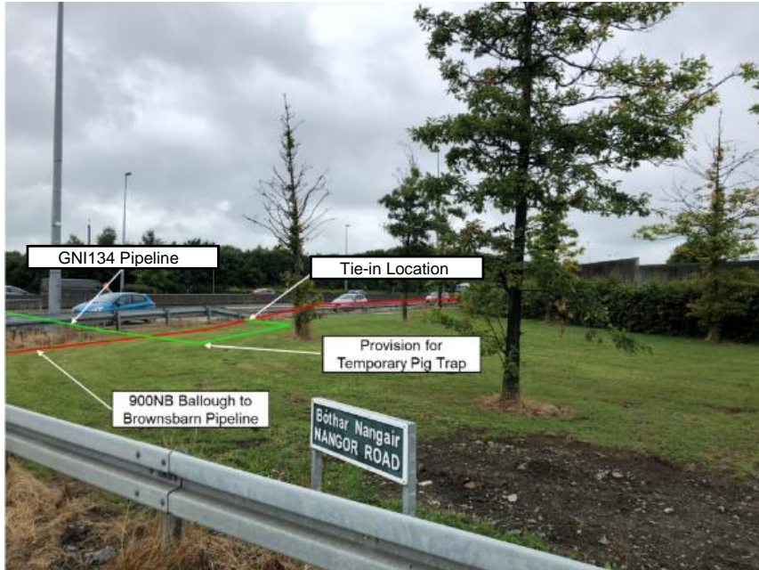
Figure 9 - Tie-in Location Street View
