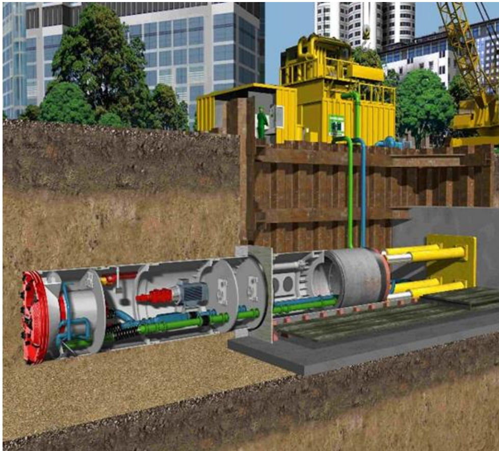
Figure 8: Conventional Closed-face Micro-tunnelling Schematic
