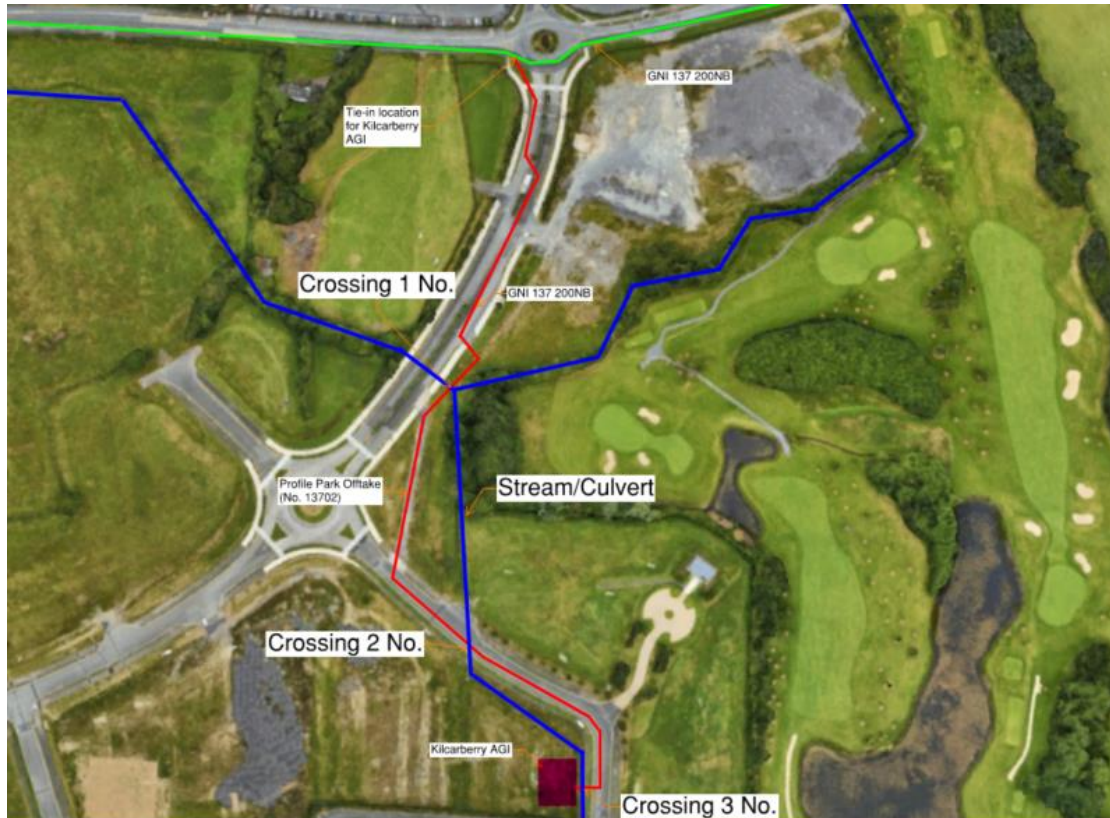
Figure 35 - Location of stream/culvert crossings
