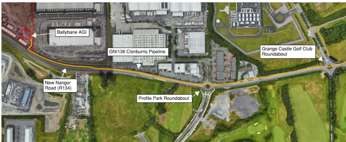
Figure 19 – Verge utilised along the north side of the New Nangor Road from the Grange Castle Gold Club Roundabout until the GNI136 pipeline enters Microsoft Operations Ireland Ltd.'s site
