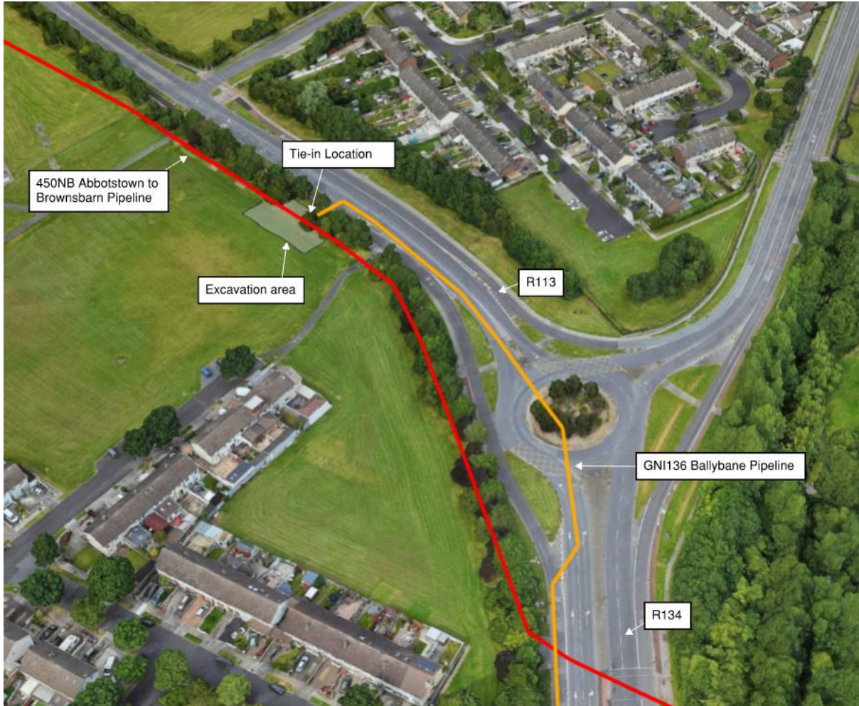
Figure 23 - Tie-in location 3D view
