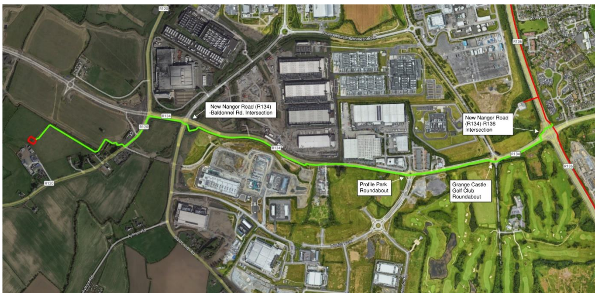
Figure 14 - Road crossings for pipeline GNI134
