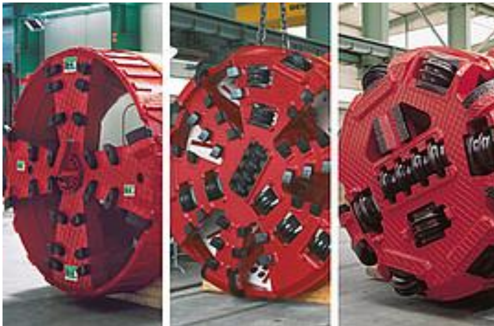
Figure 9: Conventional Micro-tunnelling Cutting Heads – Soft Ground, Mixed Ground and Rock
