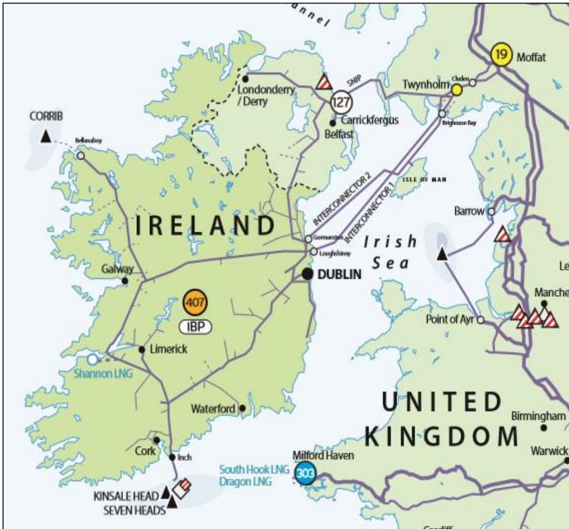
Figure 3-3 Overview of Gas System in Ireland 26
