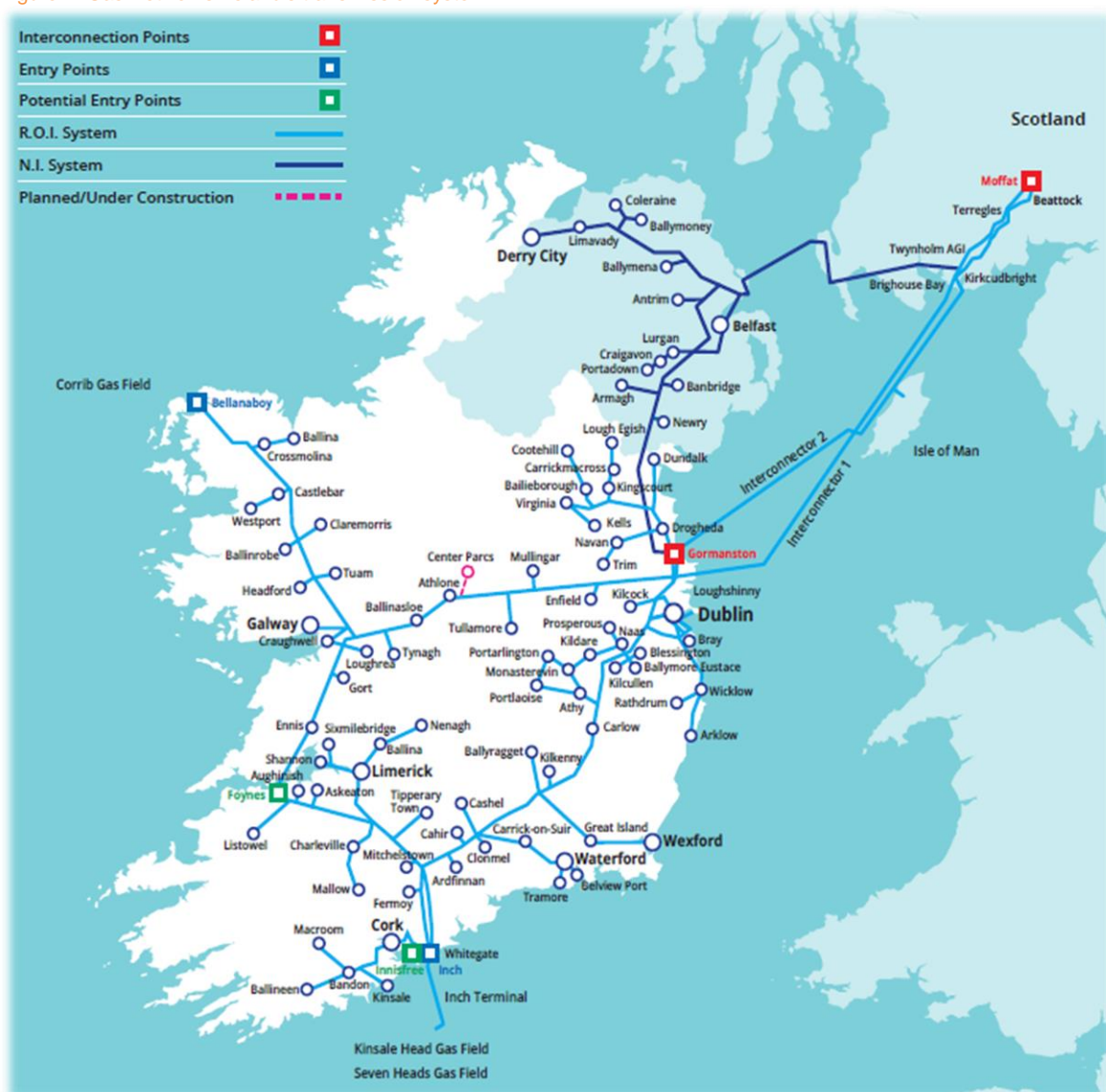
Figure 1: Gas Networks Ireland's transmission system
